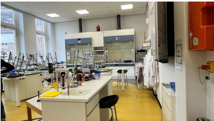
One of the chemistry classrooms; note the emergency stop button (far right) cutting off supplies
