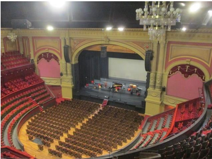
In the middle the floor can be lifted to the stage height
