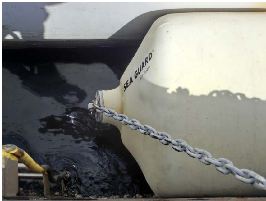
Fender with chains oriented incorrectly. Note damage to the fender ends.
