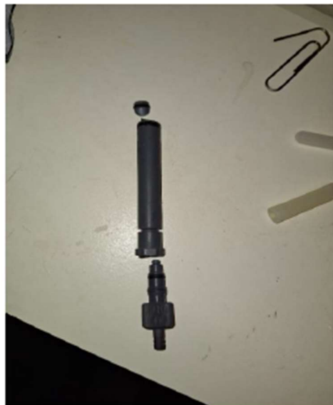
2026 - DR1 - Sample taking unit defect.
