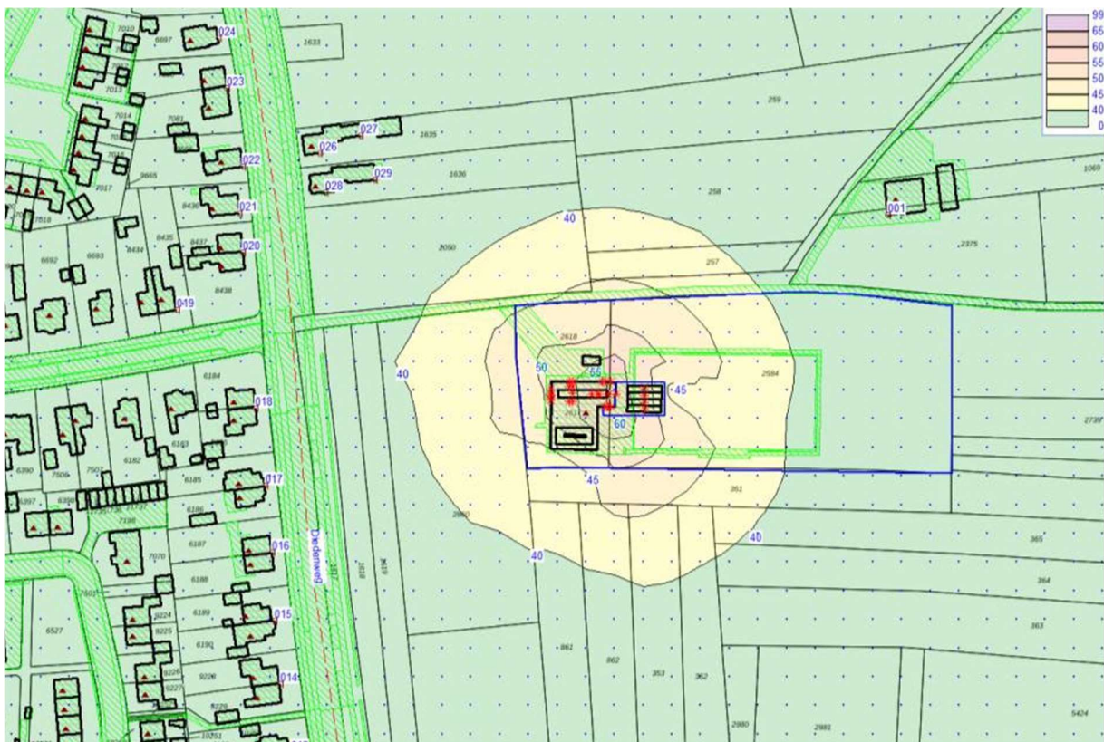
Noise contours of 40, 45, 50, 55 and 60 dB Lden, heat generation installation, applicable for the day, evening, and night periods, calculated at a height of 1 meter. 6 (source: SAB)
