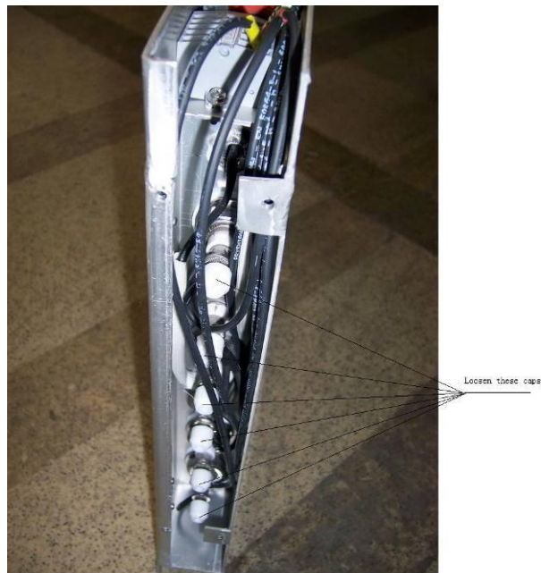
Figure 5.86 Loosen the 6 white caps
