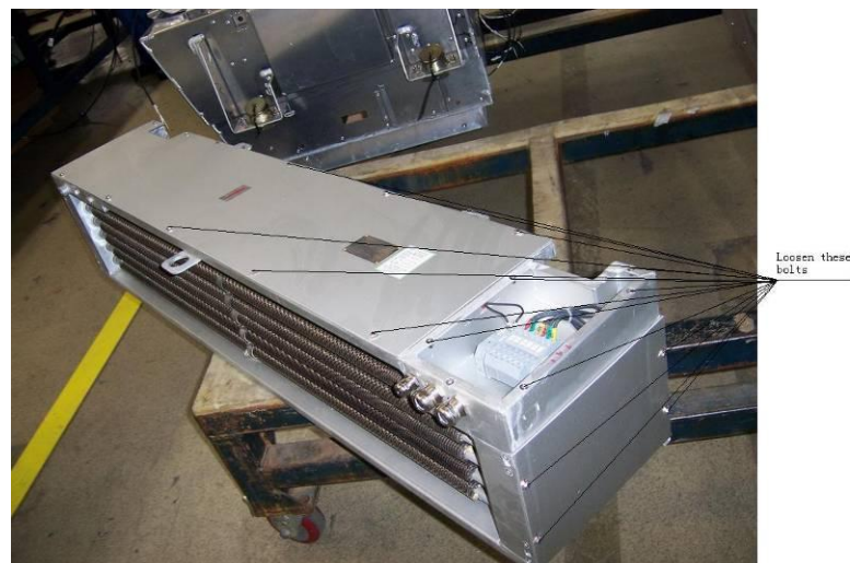
Figure 5.89 Open the heater covers
