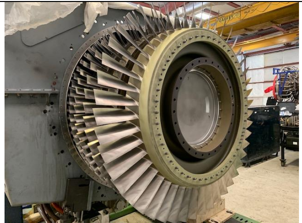
LPC rotor where dry ice cleaned
