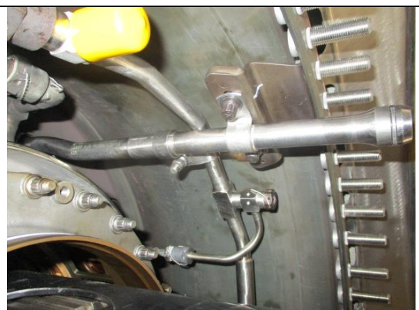
CRF oil manifold install per SB 308
