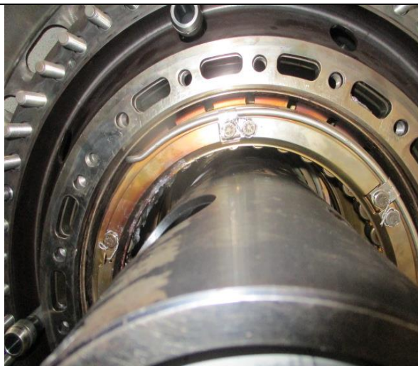
#5 bearing housing install
