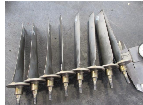
Replaced a total of 15 vanes on STG 3 upper and lower cases
