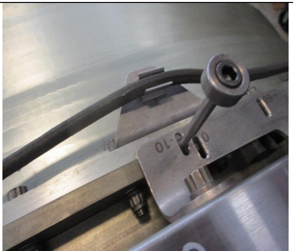
VIGV pinned at closed position
