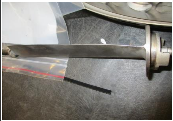
Damaged HPC Vane Lower Case stg2
