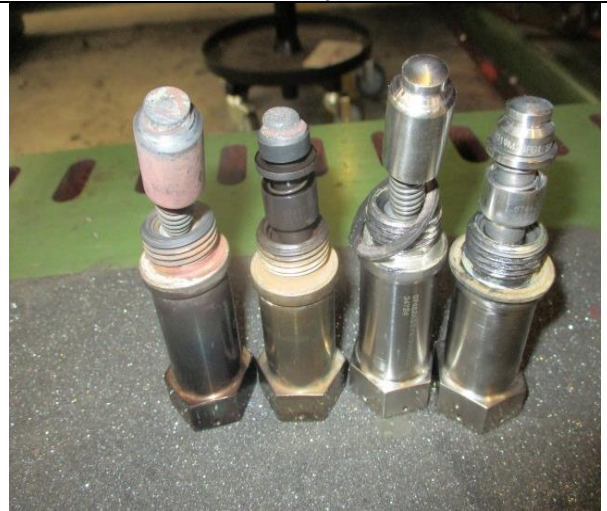
STG 1 and STG 2 plugs replaced due to wear on tip
