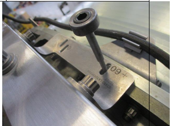
VIGV pinned at open position
