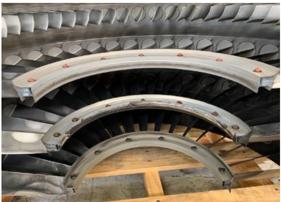
Missing Teflon and seal delamination
