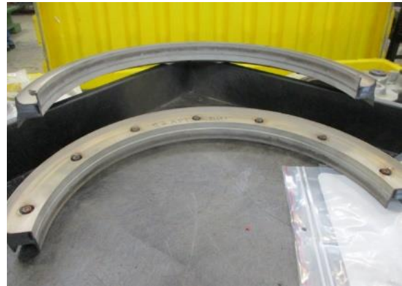
Missing Teflon and seal delamination
