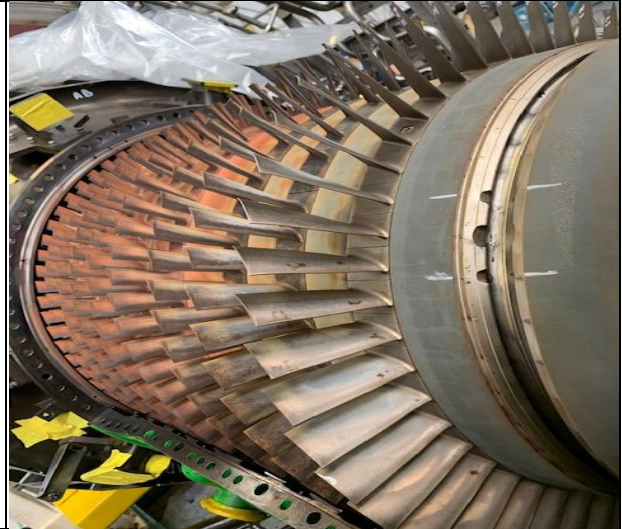
HPC rotor blades where dry ice cleaned
