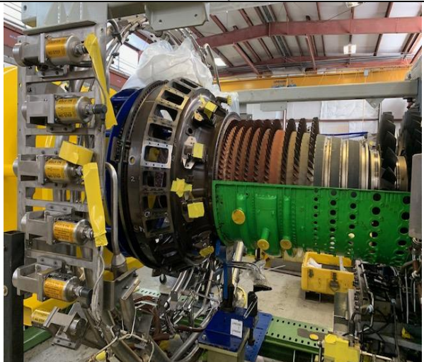
HPC rotor blades where dry ice cleaned
