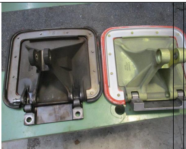
VBV doors replaced with new
