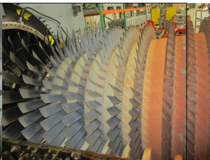
HPC rotor blades where dry ice cleaned
