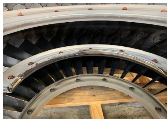
Missing Teflon and seal delamination
