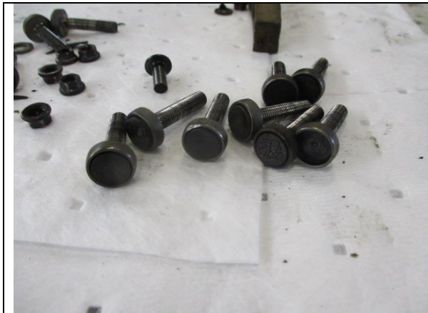
STG 3-5 rub button replaced with new
