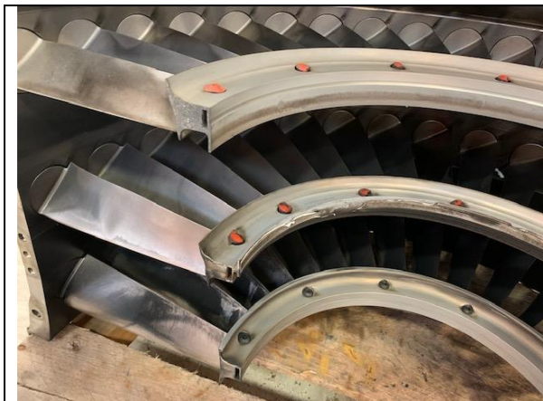
STG 2 and STG 2 shrouds replaced with new
