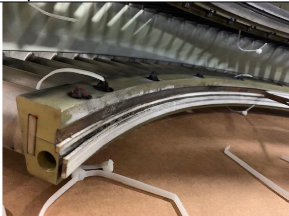
STG 3 shroud replaced on upper case
