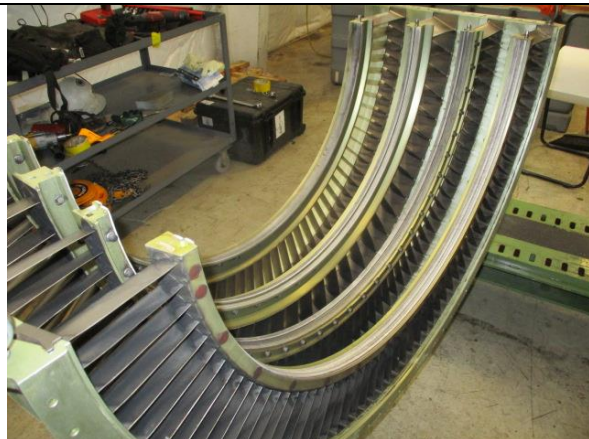
STG 3 shroud replaced on upper case
