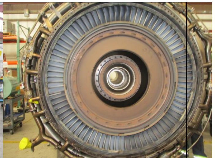
LPT with TRF Rotable LPT install
