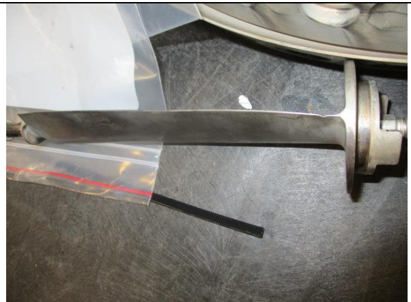
Replace one vane on STG 2
