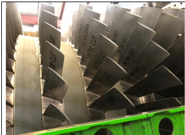
Replaced STG 3-5 blades per SB 310
