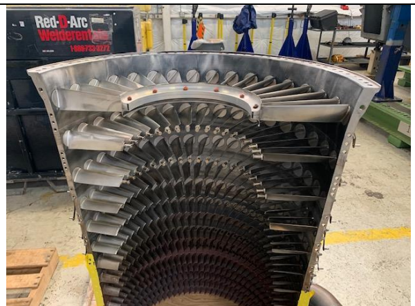
STG 2 and STG 2 shrouds replaced with new
