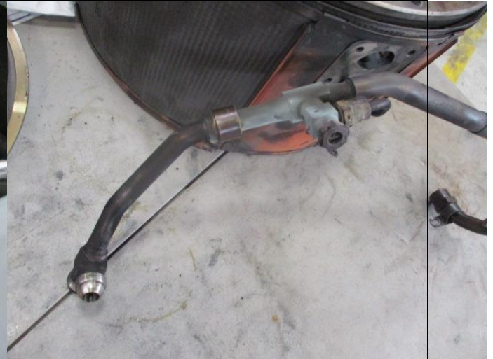
CRF oil manifold removal per SB 308
