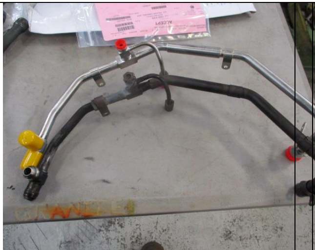
CRF oil manifold install per SB 308
