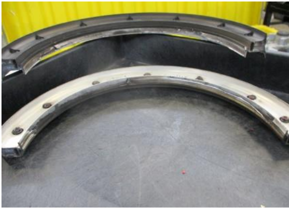
Missing Teflon and seal delamination
