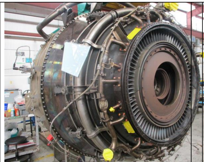
LPT with TRF Rotable install
