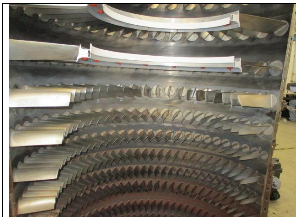
STG 2 and STG 2 shrouds replaced with new
