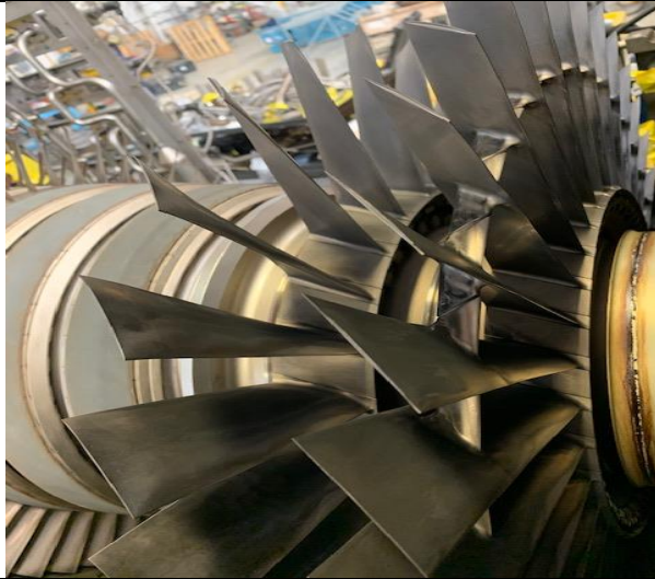
HPC rotor blades where dry ice cleaned
