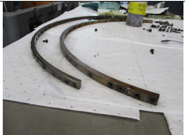
STG 3-5 rub button replaced with new
