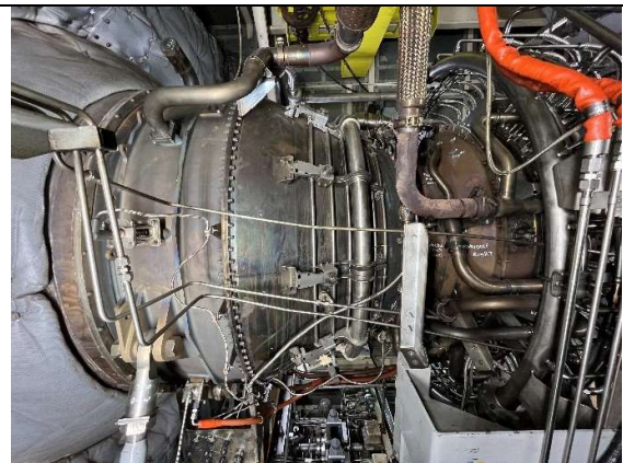
Oil found at RH side Leg, couldn't see were it is coming from.
