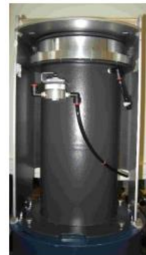
Figure 7 and Figure 8: As a good solution for this site at NFI (with also these high horizontal vibrations) we like to offer again the API dampers (Air Piston and Damped Isolators) or Gimbal dampers from TMC, which reduces vibrations in vertical and also in horizontal directions.
