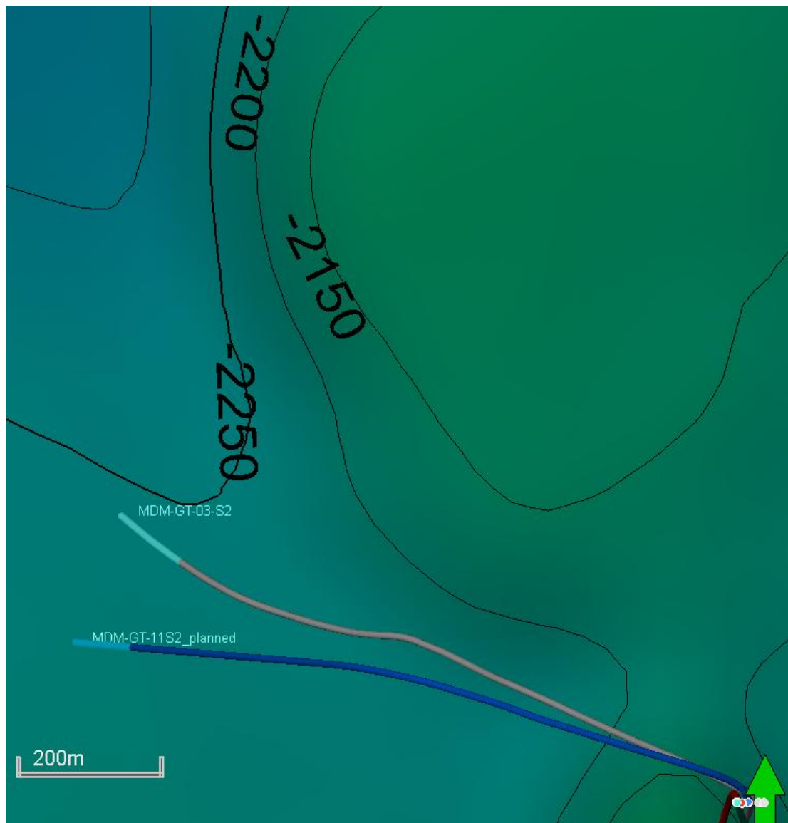
Figure 2 Close up of well MDM-GT-03-S2 and planned MDM-GT-11-S2 cutting through the top Slochteren.
