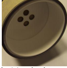
Figure 4.1 – Prototyped cylindrical mixing chamber constructed out of MCPET including 4 uniform lambertian light sources created by partially covering a remote phosphor LED module with an MCPET baseplate.
