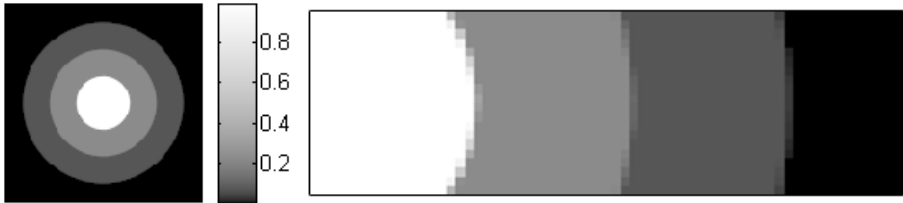
Figure 2.6 – Left: Normalized luminance map generated with the reverse ray tracing module from TracePro® (resolution: 128x128 pixels). Right: Magnified part of the luminance map.
