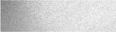
2. Bead Blasted Aluminum - for the ball tray
