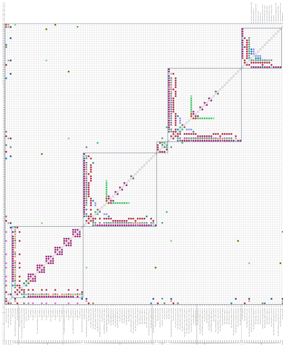
Figure 5.1: component dependency matrix of decomposition level 2.
