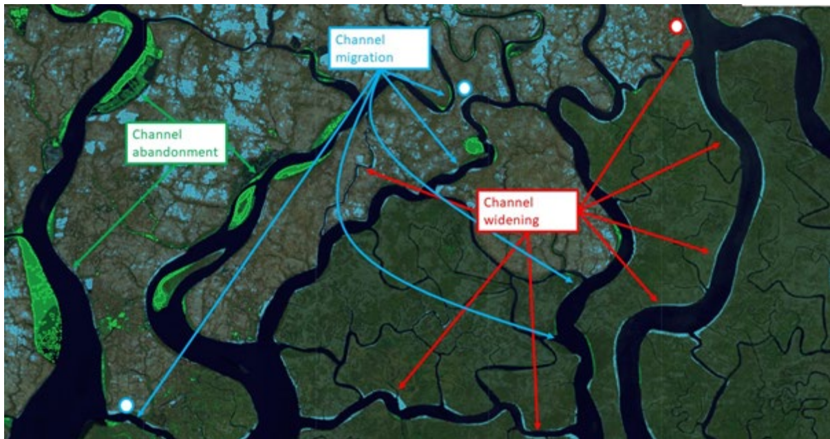
Figure 2-5. Indicative channel dynamics based on the Aquamonitor ( www.aqua-monitor.appspot.com ) in the area visited from 17-20 April. Green areas / riverbanks indicate accretion between 1990 and 2020; blue areas indicate erosion (or in case of embanked areas: land that was dry in 1990 but was covered by stagnant water such as ponds in 2020). The arrows point to areas with channel abandonment (green), channel migration (blue) and channel widening (red). White circles denote location of site visits (with the edge colour indicating the type of erosion).
