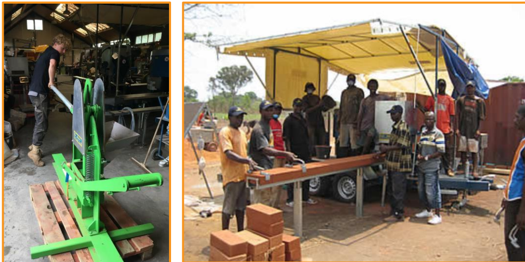
Figure 10 Hand press (l) and mobile unit (r) (Oskam V/F)
