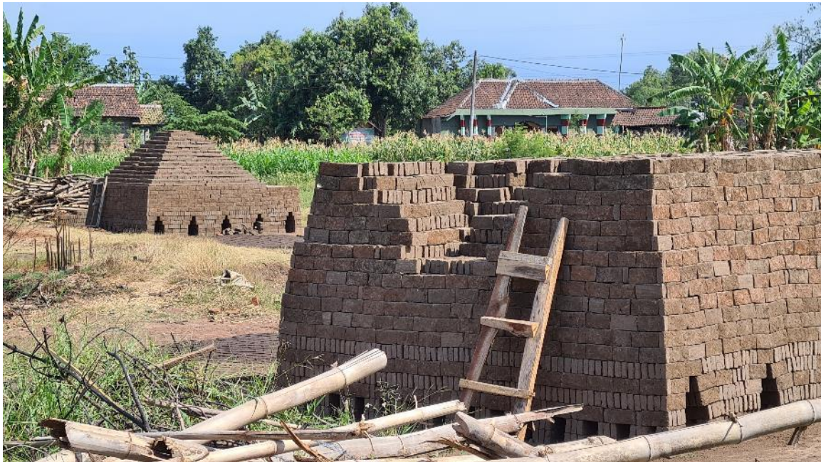
Figure 4.14 Local brick making from river sediment
