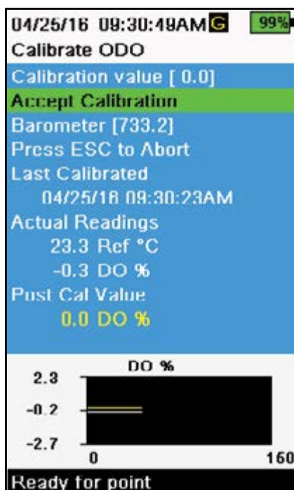
Figure 36 Calibrate DO zero point
