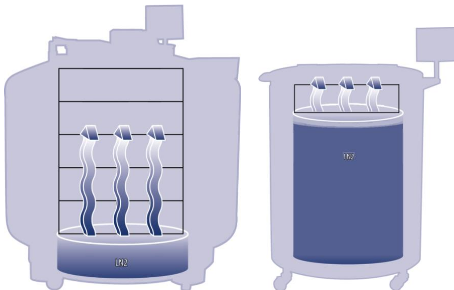
Figure 3: Illustration showing LN2 as the refrigerant. Left: LN2 below the storage space naturally boils off and cools the freezer. Right: LN2 resides in the freezer storage space.
