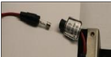
Figure 6 - Battery Backup Fuse
