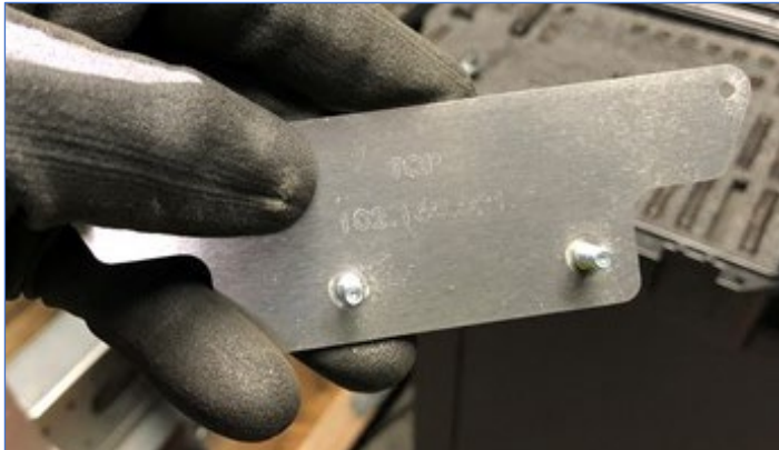
Figuur 3-10: Front TFT Mount Right Assembly
