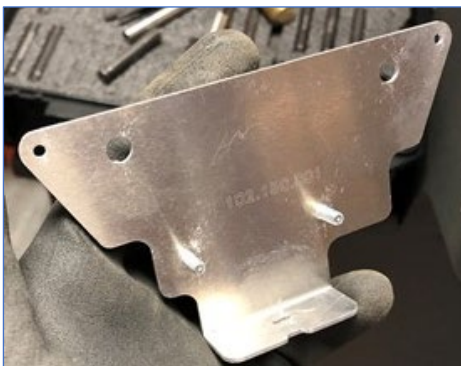
Figuur 3-9: Front TFT Mount Left Assembly
