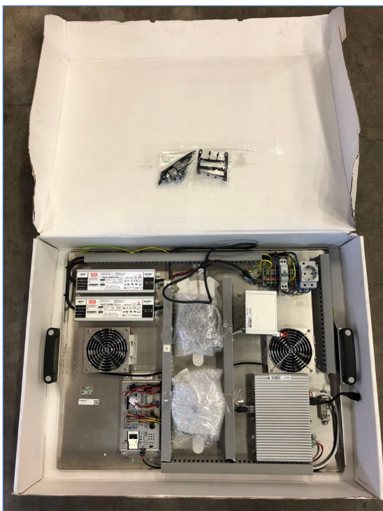
Figuur 4-1: PRES46FYT Control Assembly (Master) in doos
