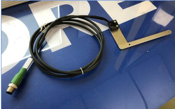
Figuur 3-7: Front Screen Light Assembly
