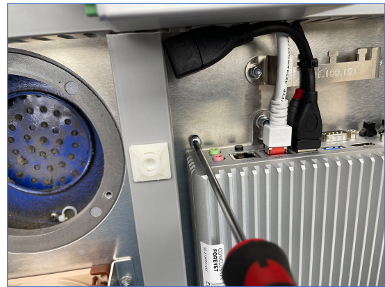
Figuur 6-5: Control Assembly bevestigen (detail)
