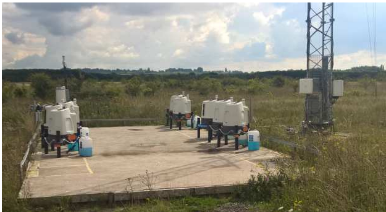
Figure 3: Typical setup of ZephIR Lidars next to the reference mast at Pershore.
