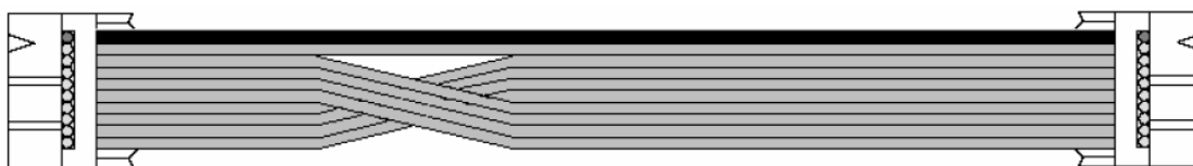
Figure 56 Cable from backpanel to I/O1609/A
