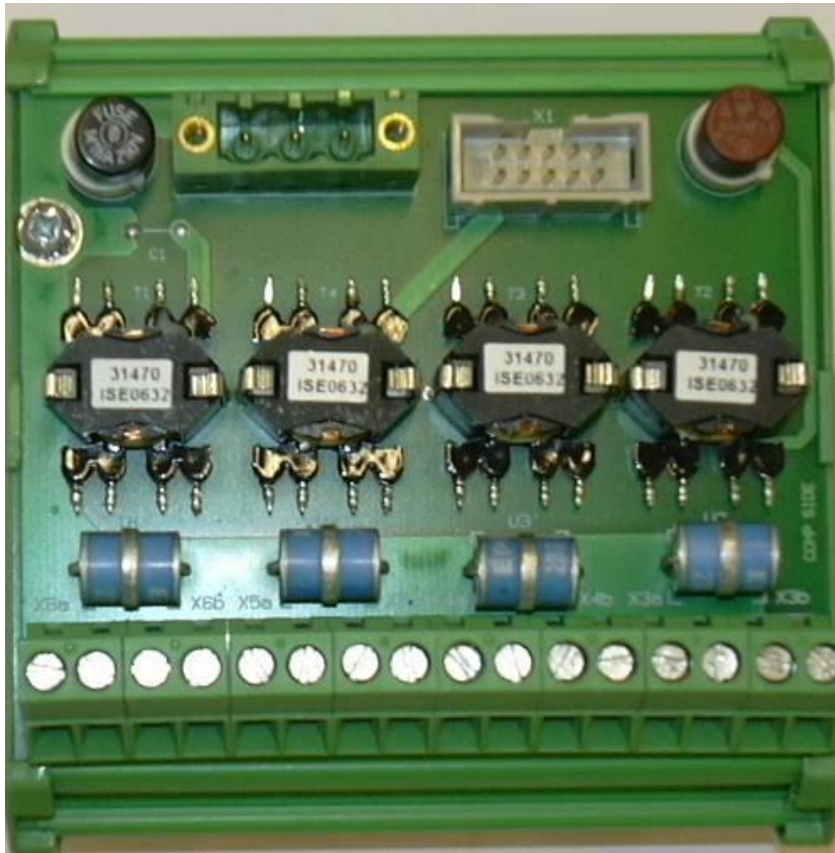
Figure 48 Loop distribution panel (LDP-T)
