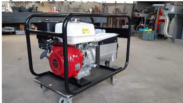
Aggregaat in frame LxBxH = 900x600x600 mm
