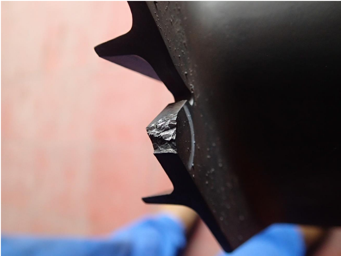
New damage 3 rd stage Bucket
