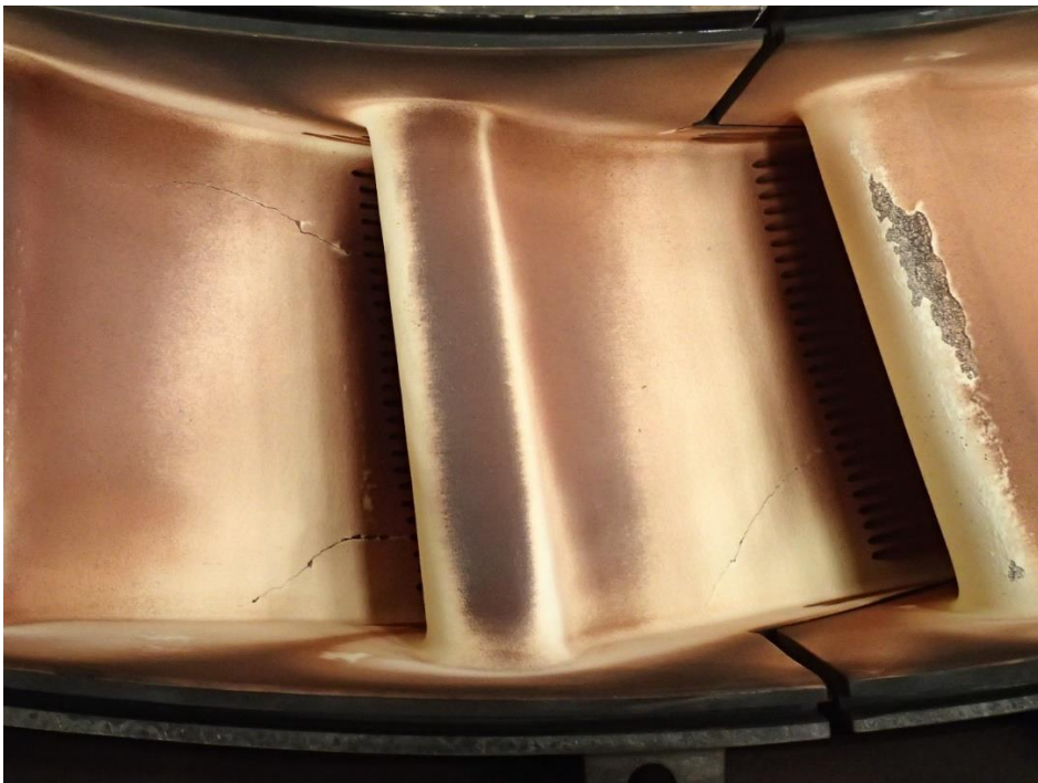
Medium Cracks on 1 st Stage Nozzle partition
