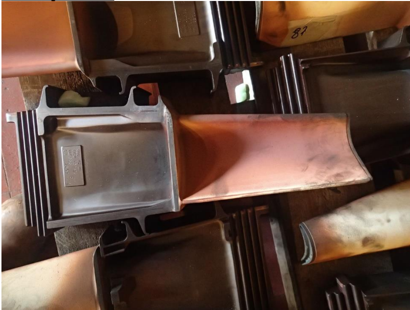
Removed 1 st stage Buckets
