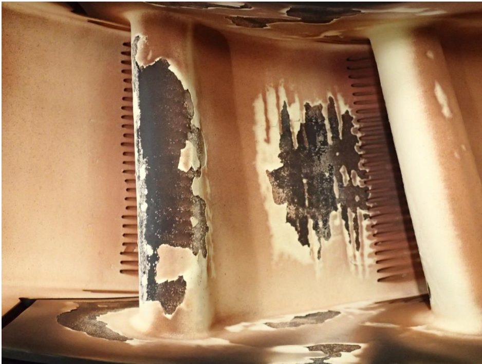
Massive Loss of TBC on Leading Edge
