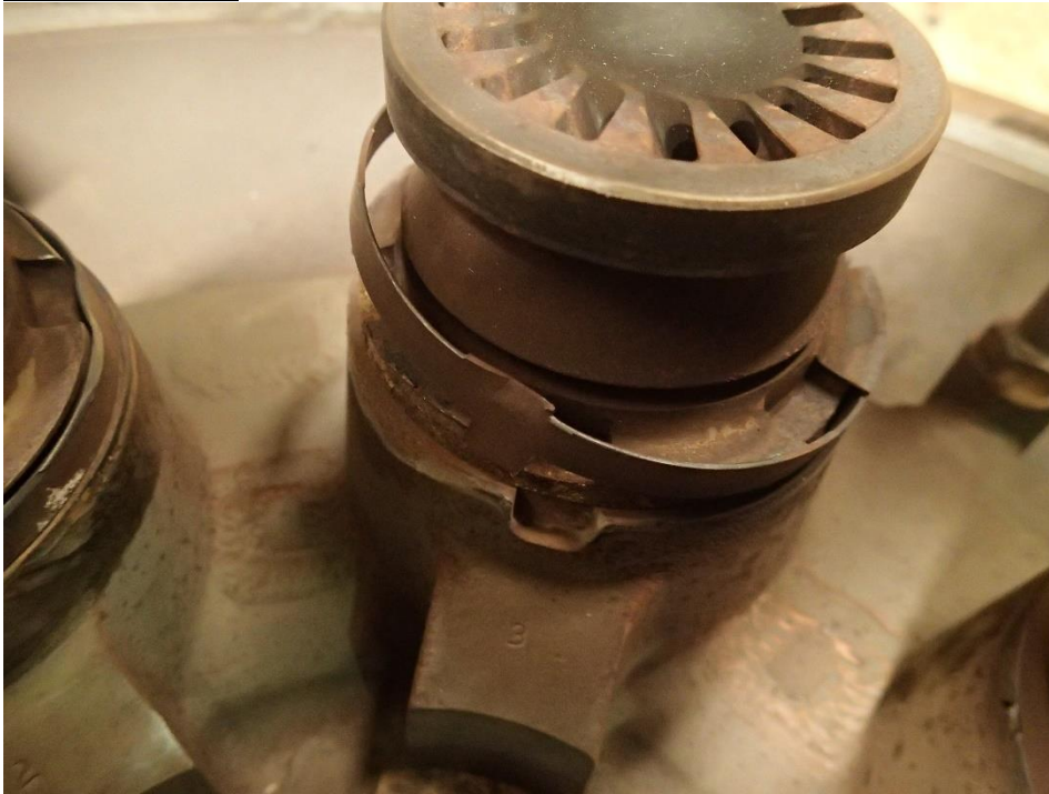
Loose Locking Ring Primary Burner
