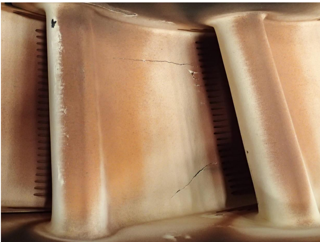
Cracks on Leading Edge
