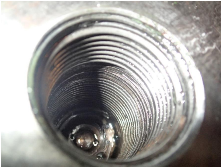
Damaged Thread Bearing #1
