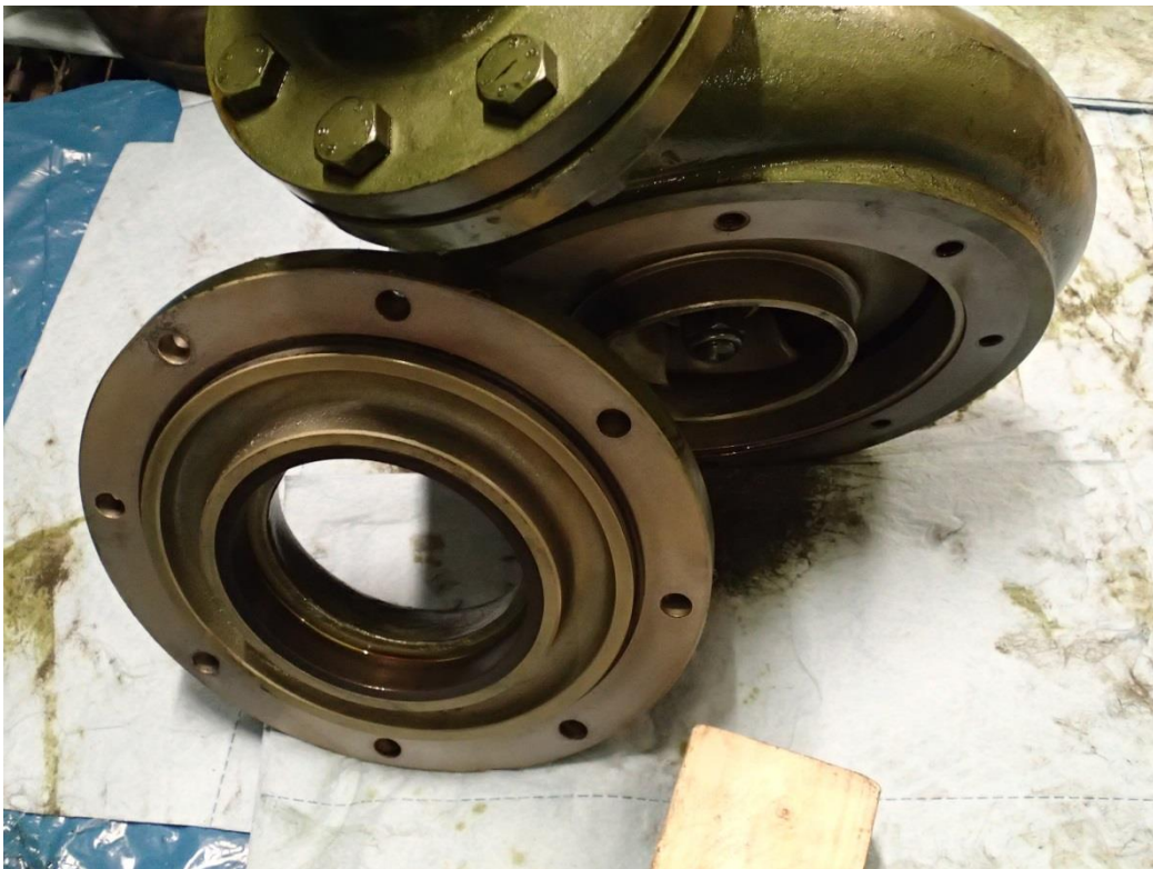
Emergency Lube Oil Pump
