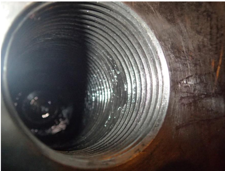
Another Damaged Thread Bearing #1
