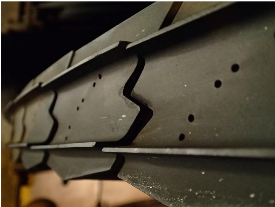
Deflection of Z-Notches 2 nd stage Buckets
