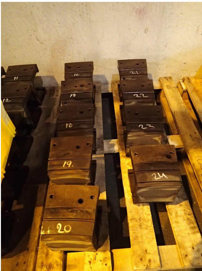
Removed 1 st Stage Shrouds
