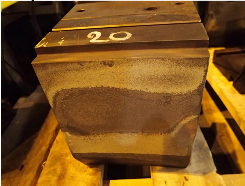
Light Erosion of TBC
