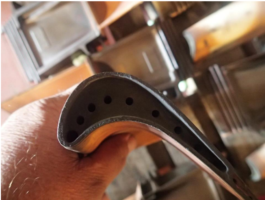
Some Minor Damage of Squealer Tip
