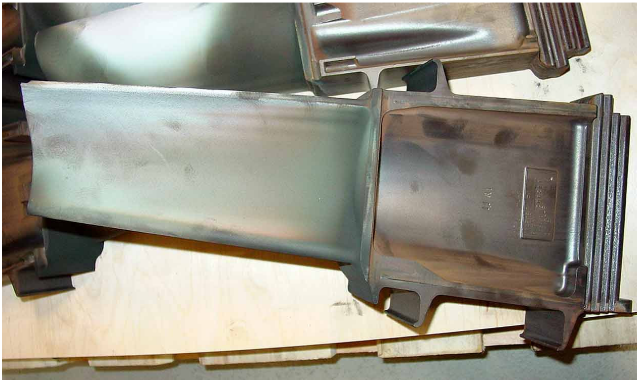
STG1 BUCKET DISCOLORATION AND HOT SPOT
