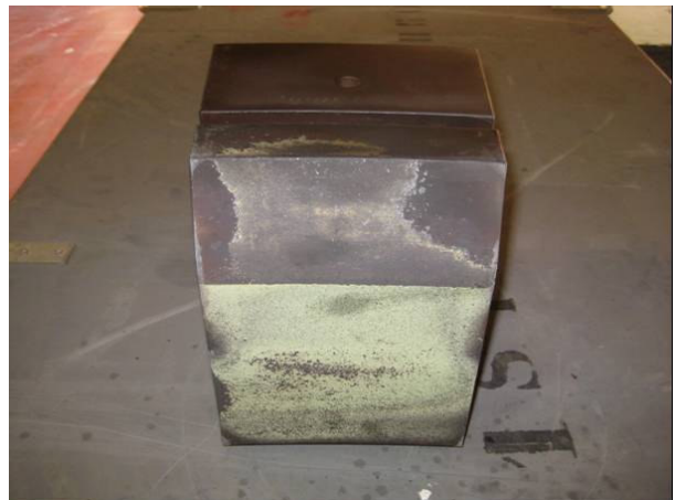
STAGE 1 SHROUD BLOCK ABRADABLE COATING GONE PLUS EVIDENCE OF AFT FACE OVERHEATING
