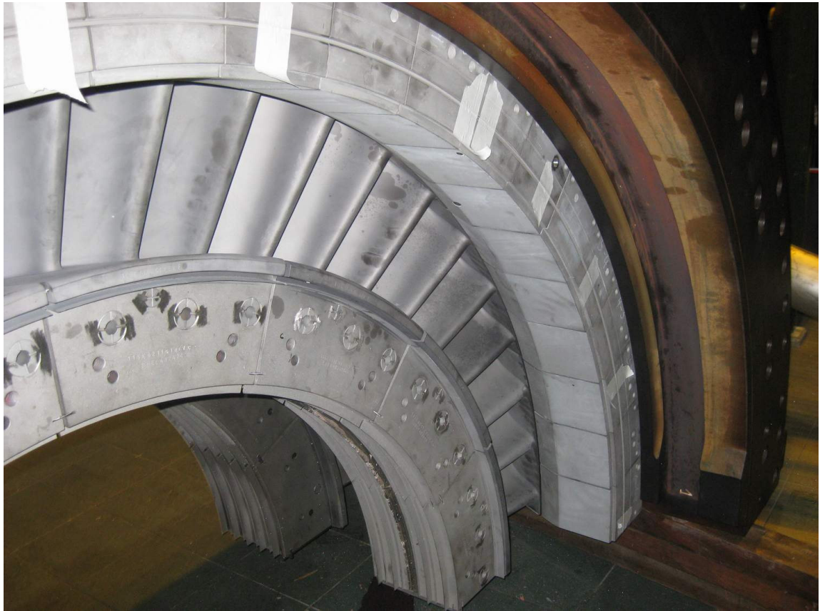
NEW HARDWARE INSTALLATION WITH PRESSURIZED W SEAL IN PLACE
