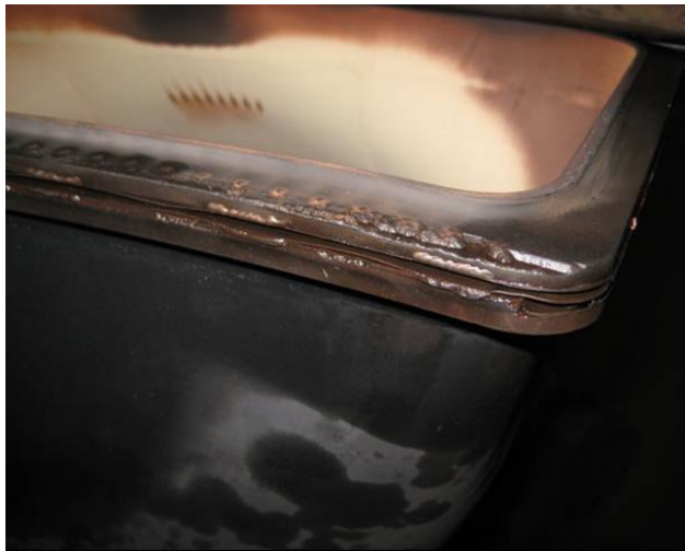
FLOATING AND SIDE SEAL SLOT HEAVY RUB EVIDENCE
