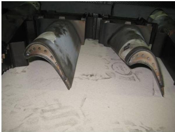
STG1 BUCKET TIP RUBBING AND GENERAL CONDITION
