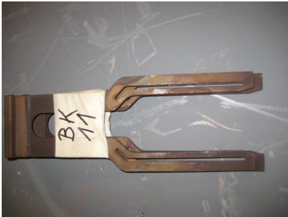
INNER CROSS FIRE TUBE RETAINER GENERAL CONDITION
