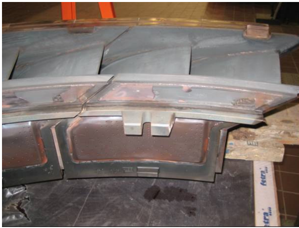
STAGE 1 NOZZLE IMPINGEMENT PLATE MISSING MATERIAL HEAVY CRACKS
