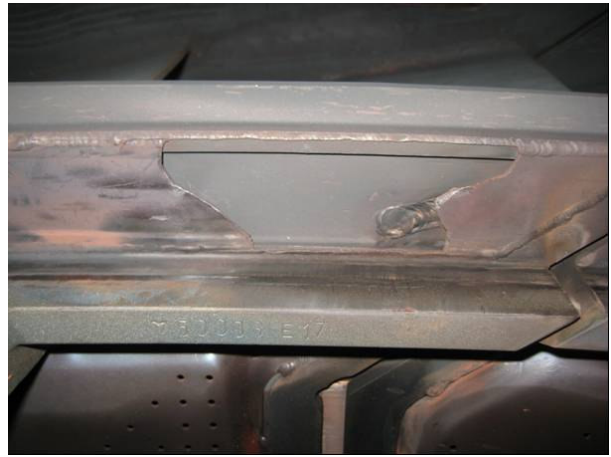
STAGE 1 NOZZLE IMPINGEMENT PLATE MISSING MATERIAL HEAVY CRACKS
