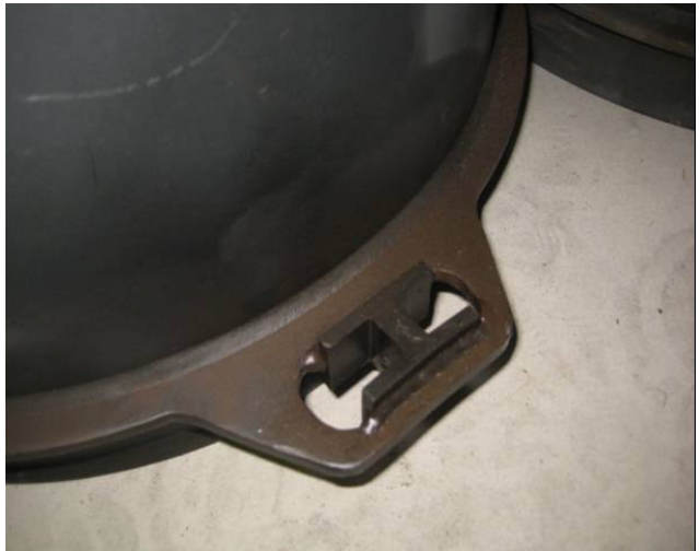
FLOATING AND SIDE SEAL SLOT HEAVY RUB EVIDENCE
