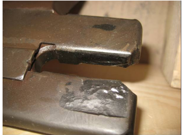
BULLHORN TYPICAL FRETTING WEAR
