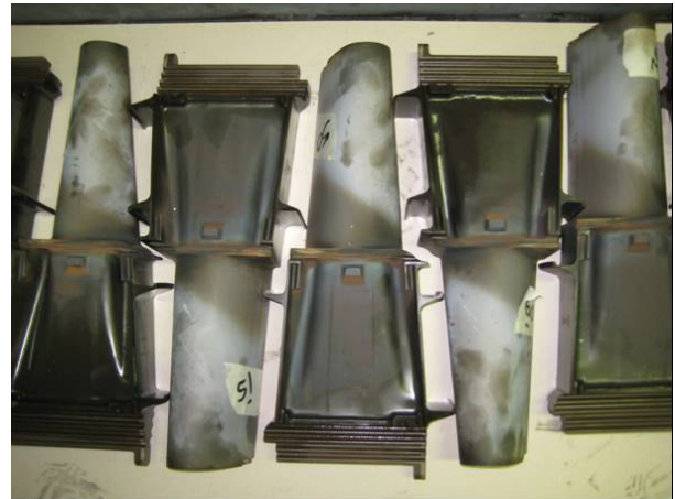
STG1 BUCKET TIP RUBBING AND GENERAL CONDITION
