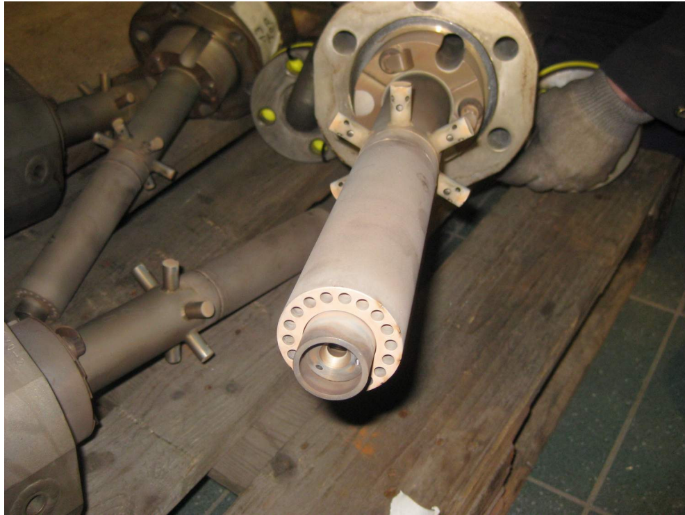
SECONDARY GAS FUEL NOZZLE WITH LIGHT CARBON DEPOSIT AND DISCOLORATION ON ITS TERTIARY TIP
