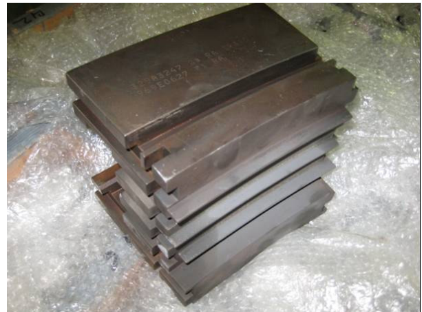
SATGE 2 SHROUD GENERAL CONDITION WITH EVIDENCE OF HOT SPOT AND OVERALL OVERHEATING
