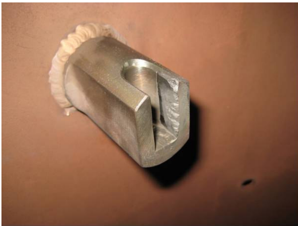
FLOW SLEEVES LINER STOPPER FIT FRETTING WEAR
