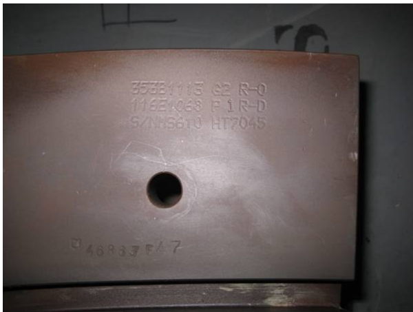
STAGE 1 SHROUD BLOCK ABRADABLE COATING GONE PLUS EVIDENCE OF AFT FACE OVERHEATING
