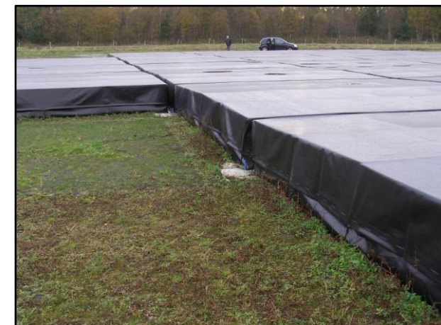
LOFAR High Band Antenne (HBA) 5x5 meter
