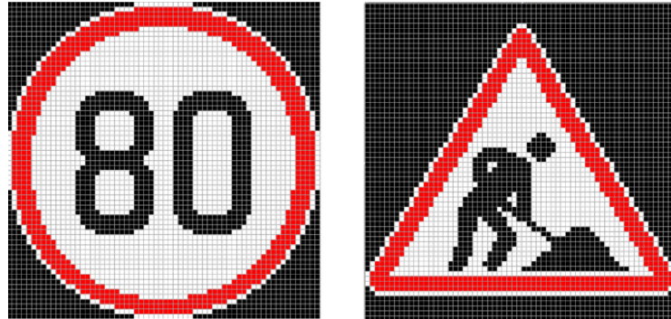
Figure M.8 — Example of VMS using (64 \times 64) elements, no colour inversion
