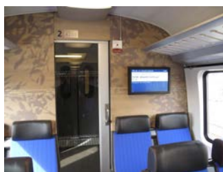
Compartment separation with sliding door
