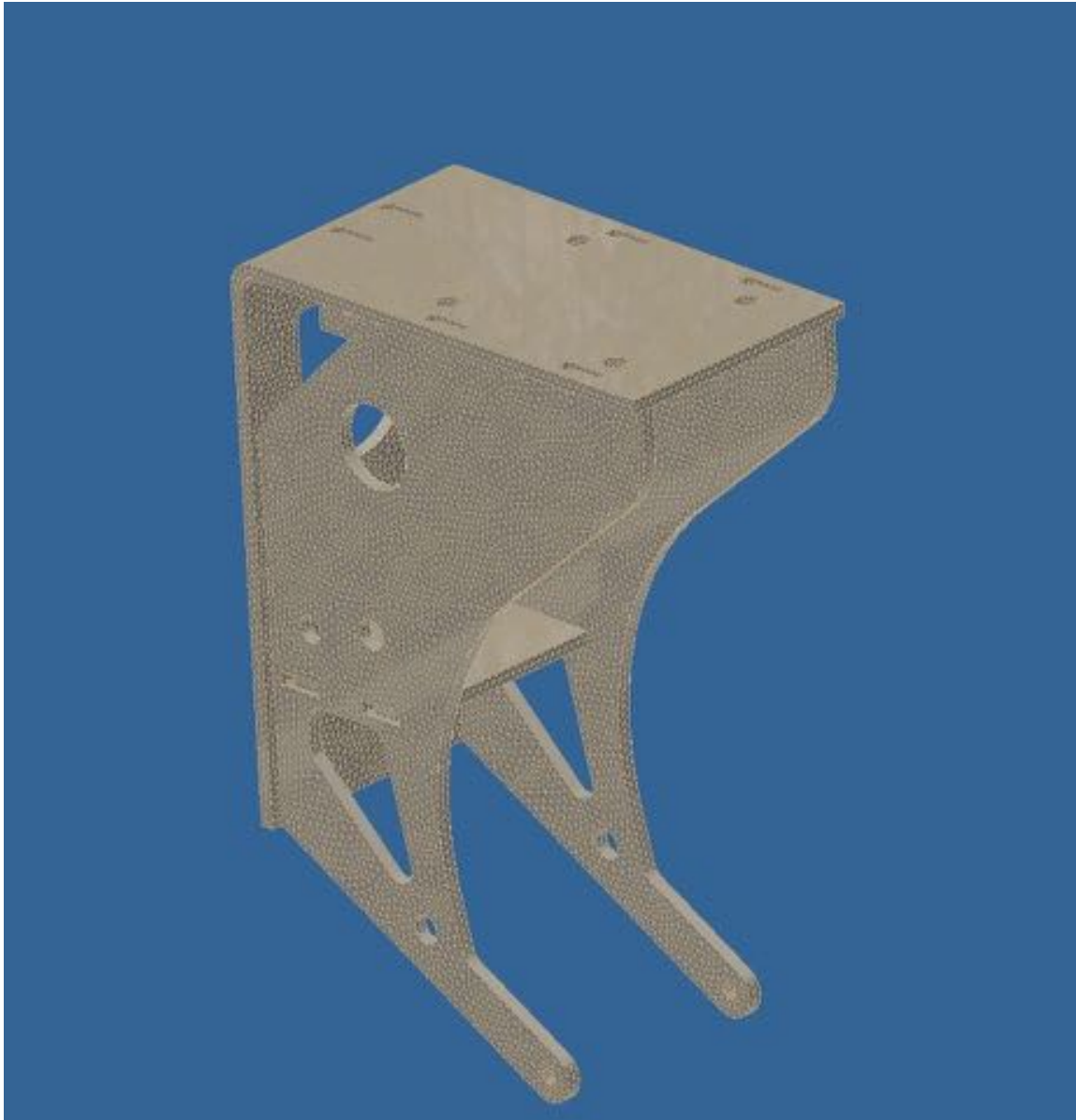
Figure 2 - Finite Element Mesh
