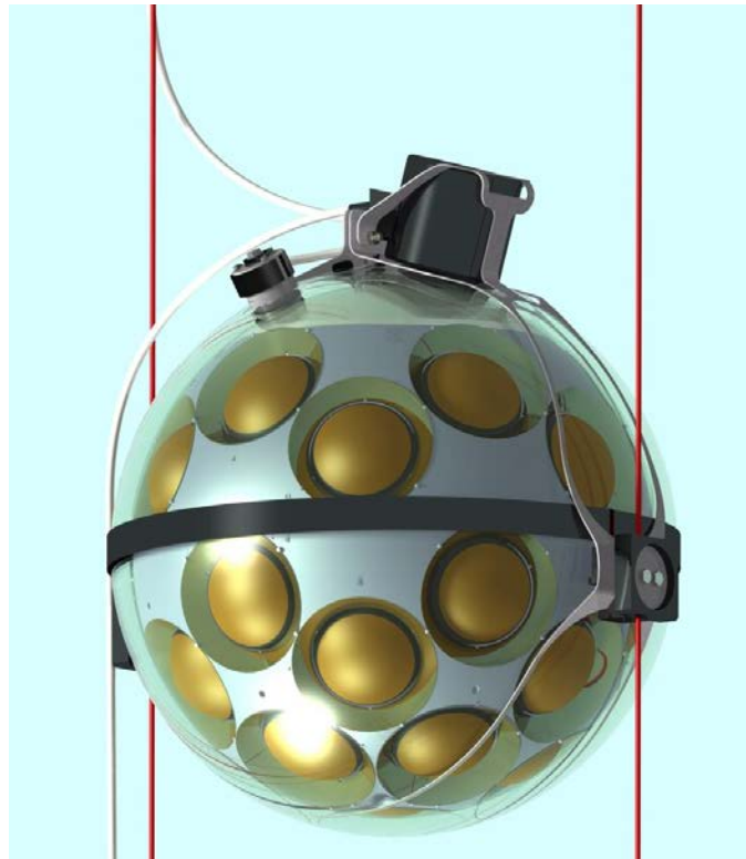
Figure 2 For information only on the use of the VEOC showing the routing of the VEOC at the DOM. A PE tube (BEOC) connects the cables coming out of the DOM through the penetrator to the DOM Breakout Box. In red Dyneema ropes that support the vertical structure of the DU.
