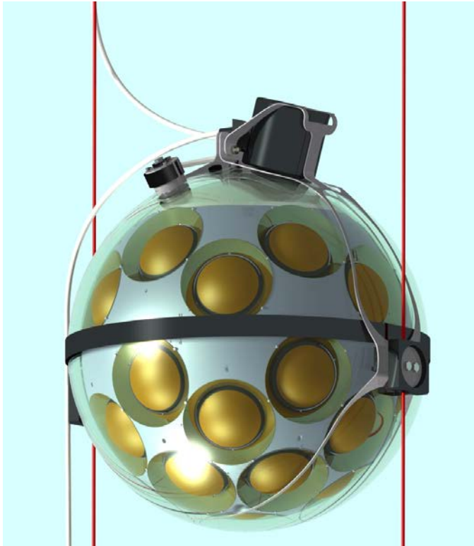
Figure 1 Routing of the VEOC at the DOM. A small PE tube (BEOC) connects the cables coming out of the DOM trough the penetrator to the DOM breakout Box. In red the Ultra High Molecular Weight Polyethylene (Dyneema) ropes that support the vertical structure of the DU.
