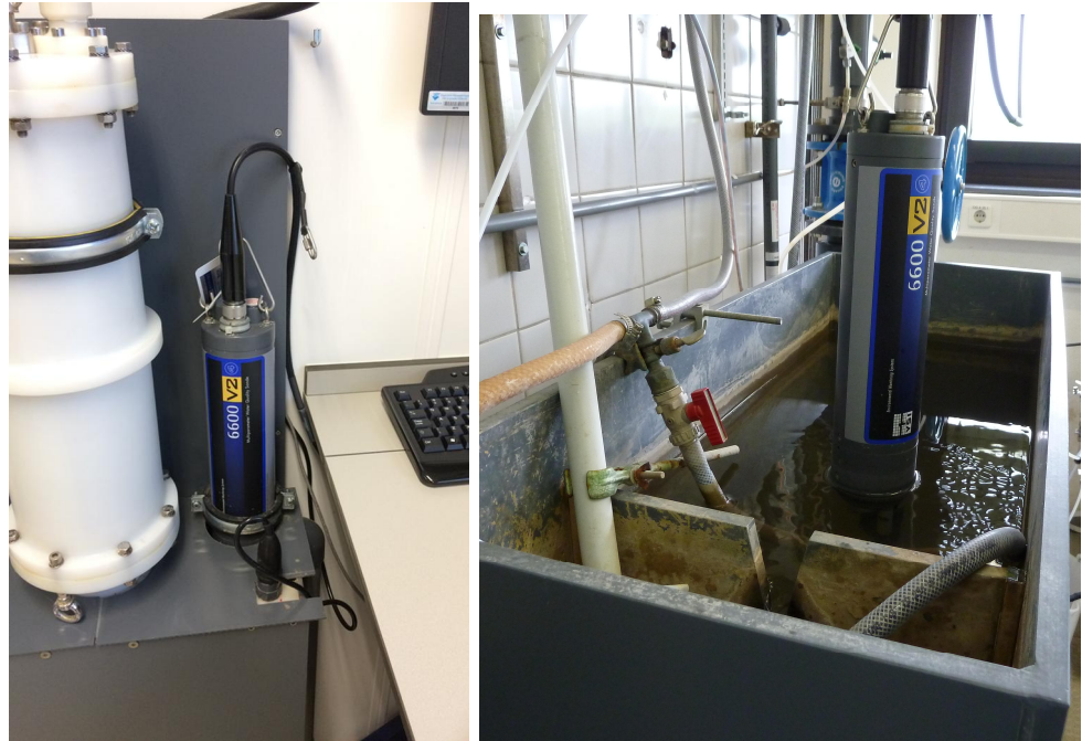
Figure 14: Application I Measuring pontoons flow-through systems (left typical for Lobith and Eijsden, right in Bimmen)
